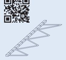
A zig-zag line is a section which allows shortterm stopping, for example for a courier, food delivery or getting on/off a vehicle, taxi, etc.
